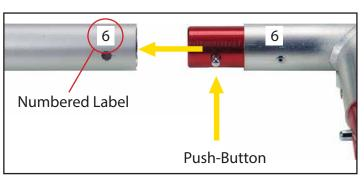
Connections are made by holding the button down and sliding the red tube into opposing tube until button locks into the hole. To disassemble, push button and pull or twist extrusions apart.
